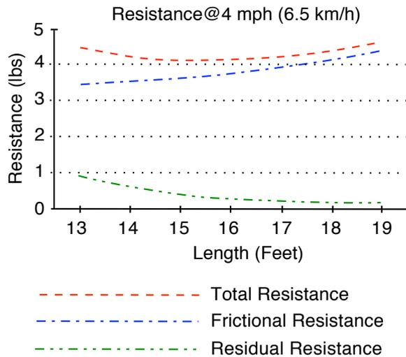
Wavemaking and frictional resistance (bottom and middle curves) are plotted for a single shape but for varying lengths. The two are added together and a curve of total resistance is drawn. You can see that the ideal length for this speed is where the curve is at its lowest point on the red line — in this case 15 feet (457 cm). Designers can choose somewhat greater length though for increased speed potential for stronger paddlers or emergency situations.
