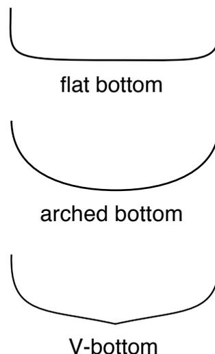
Test data indicates that the best combination is that of 'U' shaped sections at the bow, rounded sections midships, and 'V'd sections aft. The "U'd" forward sections allowing the bow paddler to make effective control strokes while the "V'd" aft sections provide directional control.
