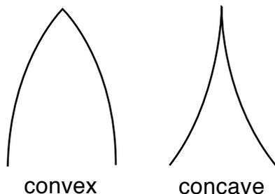
Past that point the waterline can remain full and taper to concave waterlines at the stern. If the waterlines are too concave forward the
