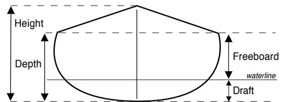
The height of the ends should normally be 1/10 of the overall length, although it is permissible to be a few inches lower in the stern. What is not shown by these dimensions is what shape the sheer profile should be. Since waves come aboard about 2–3 feet (60–90 cm) aft of the bow, the sheer should not have a sharp curvature towards the ends but rise gradually in a smooth uniform sweep.
